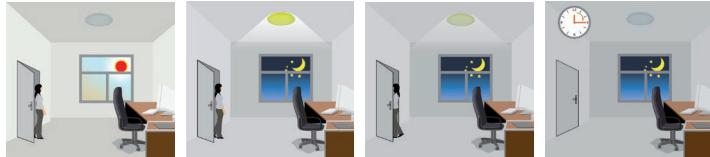
With ambient light more than daylight threshold, the lamp does not switch on when someone enters the room.
