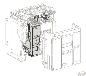
Even when the mechanism is in OFF position and discharged state, the energy spring remains under compression.
