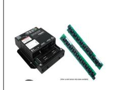
The BCPM series consists of a data acquisition board and up to 4x 21-unit current sensor strips, with 8x auxiliary inputs. The strips are mounted on each side of the panel board along the termination points of each breaker. The conductor passes through the appropriate current sensor before terminating at the breaker. Each strip transmits the current data to the data acquisition board.
