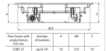
Capacity (maximum nb of modules)of floor box nr 0 88 127 depending on configuration for optimized cabling operations
