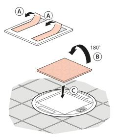
Double sided adhesive tape to fix the finishing plate on the lid & trim
