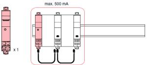
In this case is necessary to separate the two groups of devices with the decoupling white cable (delivered with the EMS CX<sup>3</sup> Power supply module)
