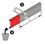
. Cut the protection plastic cover to the required length
