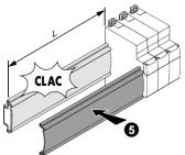
Clip the protection plastic cover on the remaining exposed part of the communicating rail
