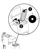
. Marked from 0 to 9 in order to locally define the Modbus address to EMS CX³ modules
