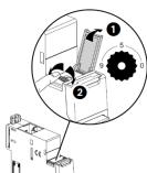
. Marked from 0 to 9 in order to locally define the Modbus address to EMS CX³ modules
