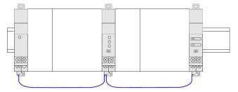
**Implementing:** with this configuration, the plastic protection cover of the backside communication ports on the EMS CX<sup>3</sup> module must be keep on.
