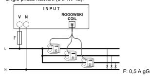
Note: the 3 single-phase circuits measured must come from the same phase.
