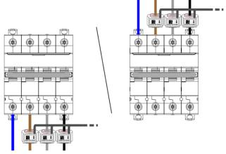
Rogowski coils must be put in the correct direction of current flow (arrow drawing on the coil).
