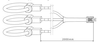
This length can be stretched via the Extension cable + connector up to 5 meters (2 m of Rogowski cable and un to 3 m of extension)
