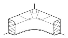
The junction in internal angle of two pieces of the same section:
