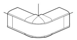
The junction in external angle of two pieces of the same section:
