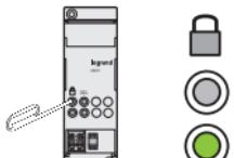
In the Scenario Module press the programming enabling pushbutton.
