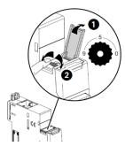
. Marked from 0 to 9 in order to locally define the Modbus address to EMS CX<sup>3</sup> modules In this system the Modbus address of an EMS CX<sup>3</sup> module device or group of modules (several functions) is obtained considering the address of the interface Modbus/EMS CX<sup>3</sup> Interface as tenth and the address of a device or group of function as unit (e.g. Interface address 1 = 10  $\rightarrow$  address of module n°5 = Modbus address 15)
