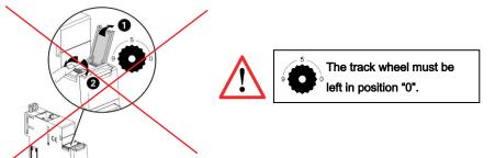
. It is not necessary to address the EMS CX<sup>3</sup> modules. The track wheel must be left in default position "0".
