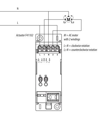
Protect with 10 A thermal magnetic circuit breaker
