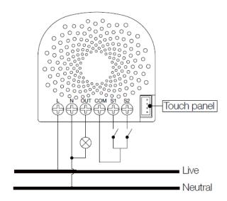
You may need to connect a small power load (E.g. a LED light or a compact fluorescent lamp) to be controlled. In this case, the Nano Dimmer may not get enough power from the AC power supply, so a bypass can be added to act as a dummy load to
