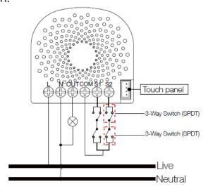
Since the S1 port and S2 port can be used to control the load separately, you can choose to connect the SPDT switches to the S1 or S2.
