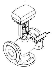
Re-mount the brace bar nuts tightening the yoke heater to the actuator and securing on to the valve.
