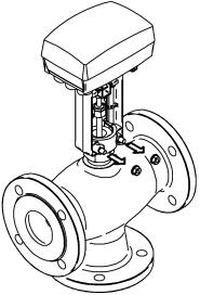
Remove the yoke brace nuts
