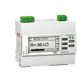
The device is a digital insulation monitoring device (IMD) for low-voltage ungrounded power systems. The device monitors the insulation of a power system and notifies any insulation faults as soon as they occur. IMD applies low-frequency AC voltage between the power system and the ground to provide accurate insulation monitoring in complex applications.
