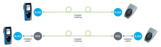
2 x M12 D connector cables supplied as standard. M12 X connectors available as accessories.
