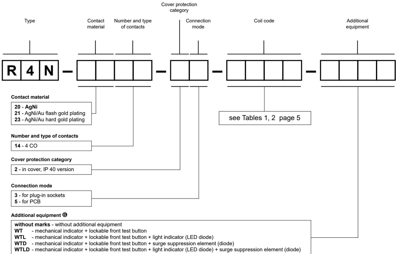
⑥ T - orange colour (AC coils), green (DC coils). WT - standard equipment of relays. WTD, WTLD - available only in relays with DC coils.
