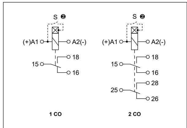
**Note:** the indicated polarization of the supply refers only to the relays RPC-...-UNI. ⚡ The control terminal S is activated by connection to A1 terminal via the external control contact S.
