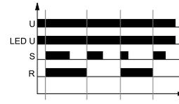
The input of the time relay is supplied with U voltage continuously. Closing of the control contact S immediately switches on the output relay R. Each next closing of the control contact S results in a change of the status of the output relay R to an opposite one (the feature of a bistable relay).
