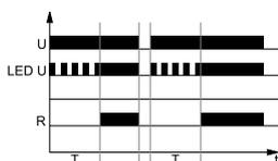
On applying the supply voltage U the set interval T begins - off-delay of the output relay R. After the interval T has lapsed, the output relay R switches on and remains on until supply voltage U is interrupted.
