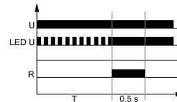
Applying the supply voltage U starts the interval T. After the interval T has lapsed, the output relay switches on for 0,5 s (the time of the NO contact of the output relay).
