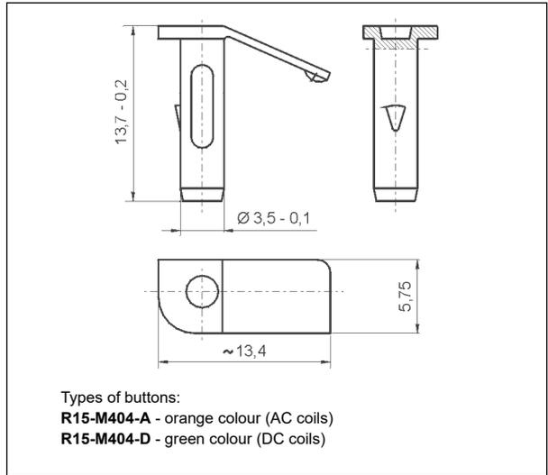
**Plugs R4W-0003** or **R15-M203** can substitute button type **T** if **manual operation (latching and testing) is not allowed**. Changing button type **T** for plug can be done by Customer themselves in the same way as changing button type **T** for button (no latching).
