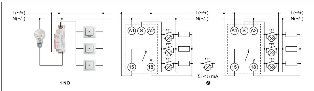
**Note:** the indicated polarization of the supply refers only to the relays RPB-1ZI-U24. Ⓢ If too many illuminated switches are connected, the lighting circuits can be switched on spontaneously or the lights can be switched on permanently.
