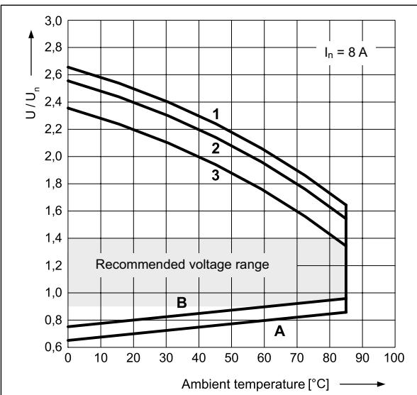
**Coil operating range - AC 50 Hz**      Fig. 5
