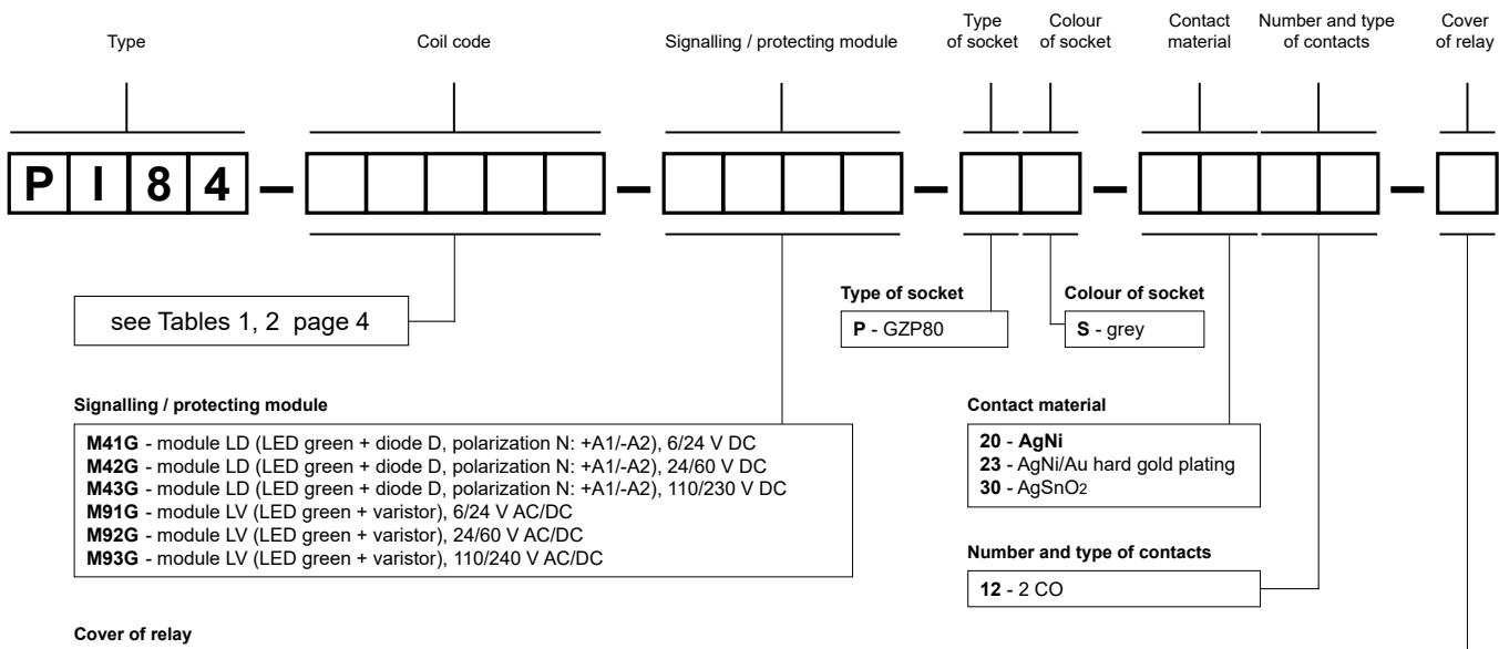
① 01: special version - relay in transparent cover, operating temperature -20...+70 °C
