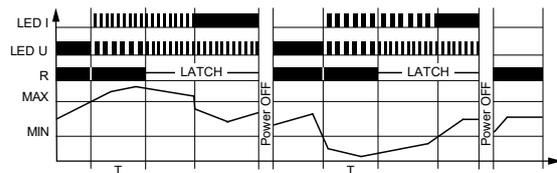
If the measured current is within the set window ( $MIN < \text{measured } I < MAX$ ), then the operational relay R is switched on. When the measured current exceeds the set window between MIN and MAX ( $\text{measured } I < MIN$  or  $\text{measured } I > MAX$ ), then after the set delay time the operational relay R will be switched off.
