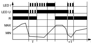
If the measured current has a value higher than MIN, then the operational relay R is switched on. When the measured current is lower than MIN, then after the set delay time the operational relay R will be switched off.
