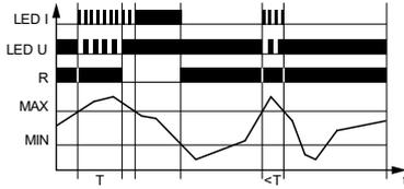
If the measured current has a value lower than MAX, then the operational relay R is switched on. When the measured current exceeds the MAX value, then after the set delay time the operational relay R will be switched off.
