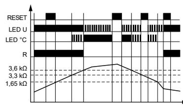
Reset by power supply voltage.
