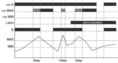
When the supply voltage U is applied, the output relay R switches into on-position, if the measured current exceeds the MAX-value. When the measured current falls below the MIN-value, the output relay R switches into off-position after the interval of the tripping delay has expired.
