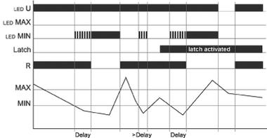
When the supply voltage U is applied, the output relay R switches into on-position, if the measured current is beyond the MIN-value. When the measured current falls below the MIN-value, the output relay R switches into off-position after the interval of the tripping delay has expired.
