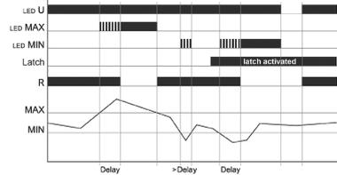
When the supply voltage U is applied, the output relay R switches into on-position, if the measured current is within the adjusted window. When the measured current leaves the window between MIN and MAX, the output relay R switches into off-position after the interval of the tripping delay has expired.
