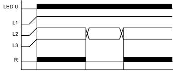
When all the phases are connected in the correct sequence and the measured asymmetry is less than the fixed value, the output relay R switches into on-position (yellow LED illuminated). When the phase sequence changes, the output relay R switches into off-position (yellow LED not illuminated).
