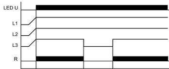
The output relay R switches into off-position (yellow LED not illuminated), when one of the three phases fails.
