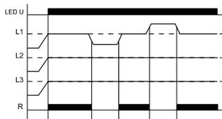
The output relay R switches into off-position (yellow LED not illuminated) when the asymmetry exceeds the value set at the ASYM-regulator. An asymmetry caused by the reverse voltage of a consumer (e.g. a motor which continues to run on two phases only) does not effect the disconnection.
