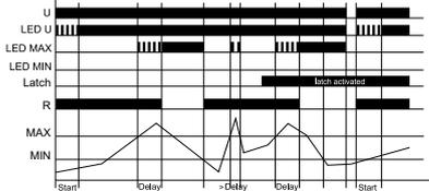
When the measured current exceeds the value adjusted at the MAX-regulator, the set interval of the tripping delay begins (red LED MAX flashes). After the interval has expired (red LED MAX illuminated), the output relay  $R$  switches into off-position (yellow LED not illuminated). The output relay  $R$  again switches into on-position (yellow LED illuminated), when the measured current falls below the value adjusted at the MIN-regulator (red LED MAX not illuminated).
