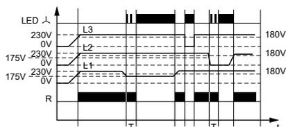
If the voltage at all phases will exceed 175 V and no error condition occurred earlier, then the operational relay R is switched on. If voltage at one of the three phases, L1, L2, L3 falls to a value of 175 V, then after applying a delay time 4 s, the R contact is switched off. The operational relay R will be switched back on when the voltage value at the given phase rises to 180 V. A rapid phase loss is treated as a phase sequence error and no delay is then applied.
