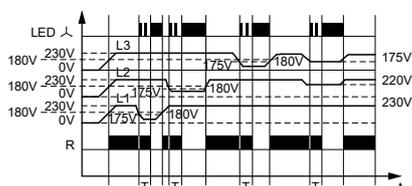
The operational relay R switches to the off position when the asymmetry exceeds the value 55 V. The asymmetry caused by the return voltage of the receiver (e.g. a motor that still operates in only two phases) does not disconnect.
