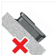
Do not mount the charging station on an inclined surface
