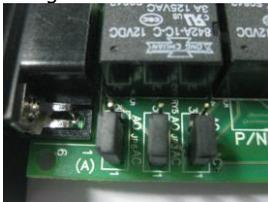
**Fig. 6 Jumper setting for ACTIVE CLOSE**
