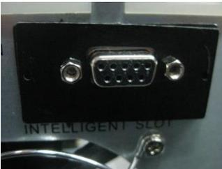
**Step 4:** Use the 9-pin communication cable to connect UPS and equipment to implement the remote monitoring and control.
