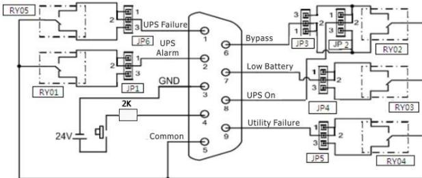
**Fig 2 Connection for ACTIVE CLOSE**
