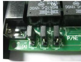
**Fig. 7 Jumper setting for ACTIVE OPEN**
