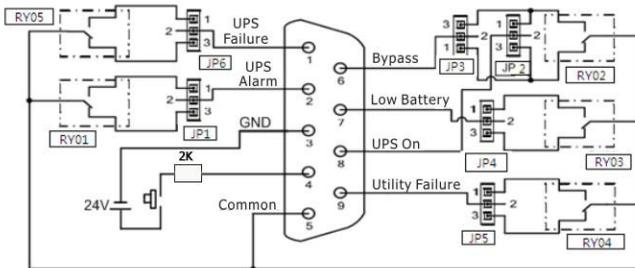
**Fig 1 Pin definition and internal logical connection**
