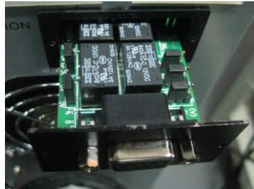
**Step 3:** The cover of AS400 should attach close to the rear panel. Using screwdriver, secure the AS400 to the UPS chassis with 2 screws.
