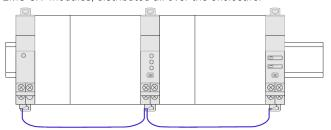
Implementing: with this configuration, the plastic protection cover of the backside communication ports on the EMS CX3 module must be keep on.
