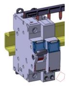
2. Pull the device forward in order to release it from the rail
