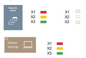
In these configurations the module can have the LEDs always off or the LEDs follow the status of the input. With this module it is possible to view and supervise the status of its inputs.
