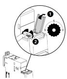
. Marked from 0 to 9 in order to locally define the Modbus address to EMS  $CX^3$  modules In this system the Modbus address of an EMS  $CX^3$  module device or group of modules (several functions) is obtained considering the address of the interface Modbus/EMS  $CX^3$  Interface as tenth and the address of a device or group of function as unit (e.g. Interface address  $1=10 \rightarrow$  address of module  $n^\circ 5=$  Modbus address 15)
