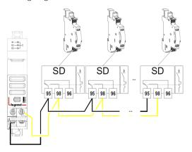
For DPX $^3$  fault contact auxiliaries use terminals 51 (instead of 95) and 54 (instead of 98) of the cat. no 4 210 11
