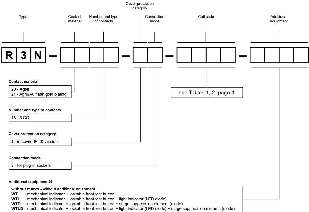
④ T - orange colour (AC coils), green (DC coils). WT - standard equipment of relays. WTD, WTLD - available only in relays with DC coils.
