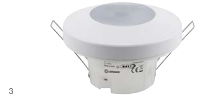
SENSOR DALI-2 LIGHT-PRESENCE-8 INFRARED CEILING INTEGRATION DALI-2 input device, infrared presence detector with 8 m movement detection
