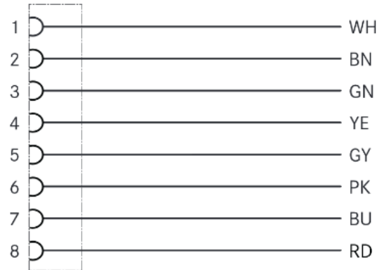
Pin assignment from M12-jack
